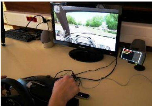
Figure 3: The study setup: the Leap motion controller is located below the hand and the IVIS display is located next to the screen of the simulator.
