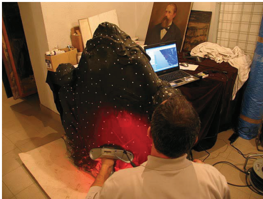
Figure 3. Laser scanning of the monument fragment
