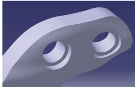
Figure 21. Creating screw holes
