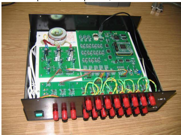
Figure 11. One practical implementation of the device - the four-channel three-phase power analyzer
