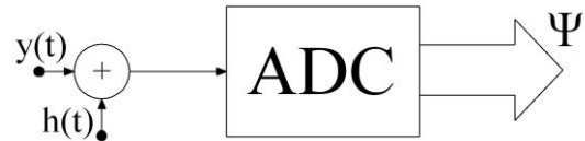
Figure 1. Block diagram of application of a uniform random dither h to the measured signal y
