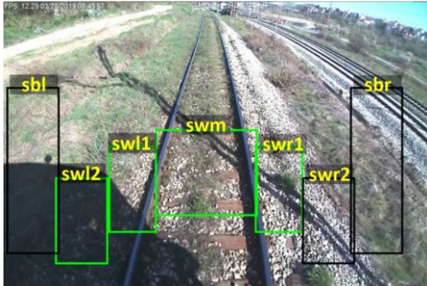
Figure 3. Position of areas for detecting weed and bushes at camera field of view
