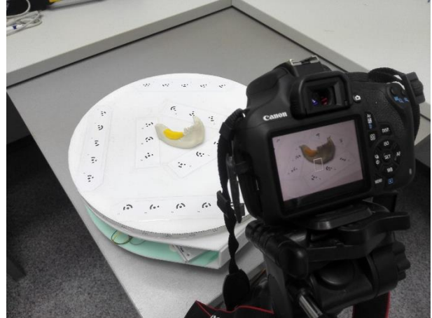
Figure 5. CRP photos acquisition setup
