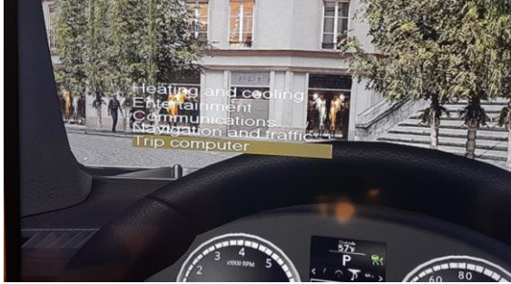
Figure 2: HUD: five lines are representing the menu items and the green bar highlights the selected element
