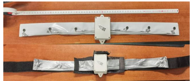
Figure 4. Pre-prototype of the wearable haptic interface for biomechanical feedback. The top image shows the exposed vibromotors with connections to the main control unit. Each motor is connected separately to the control unit. The bottom image shows the final sealed design ready for testing.
