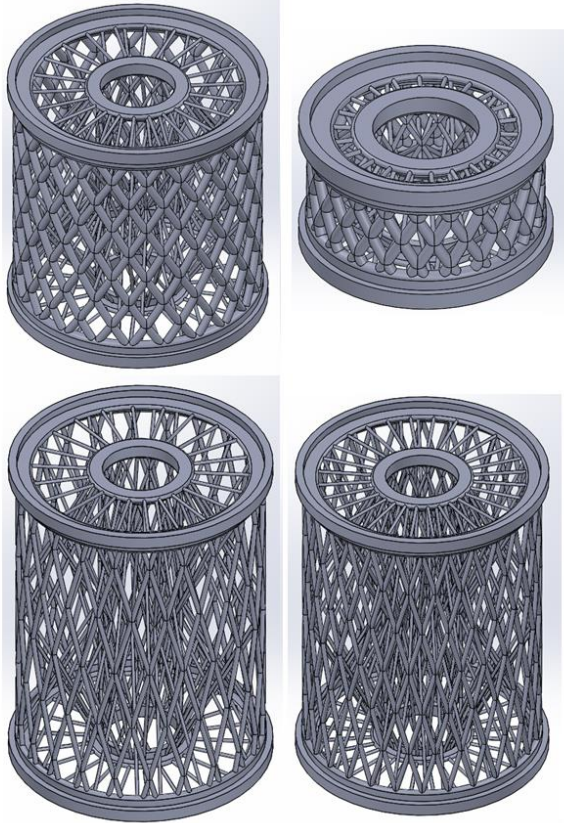
Figure 9. Different parametric sets of generic parameterized lattice scaffold model
