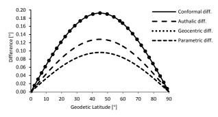
Figure 2. Auxiliary Latitudes – The divergence from the geodetic latitude
