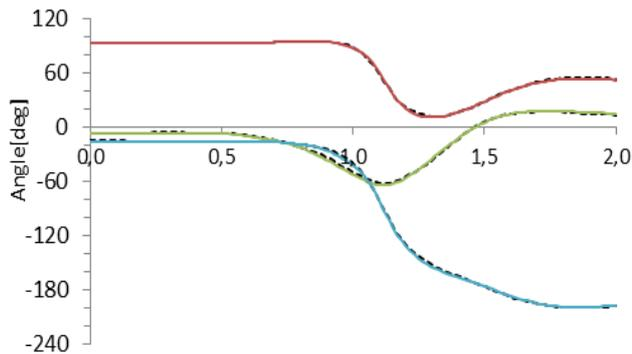
Figure 4. Comparison of smartphone embedded gyroscope (dotted black plots) and QTM body rotation angles (solid colored plots: red=roll, green=pitch, blue=yaw). Figure shows the first part of the golf swing movement in 2 seconds time interval from address to top of the backswing.
