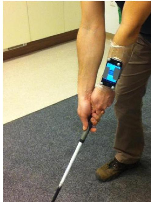
Figure 3. Experimental setup for golf swing motion. Four infrared reflecting markers are attached directly to smartphone to form the defined QTM rigid body orthogonal vector basis.
