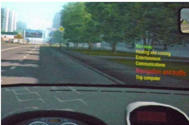
Figure 5. Driving simulator used for evaluation of auditory, visual (HUD) and multimodal interfaces [19]
