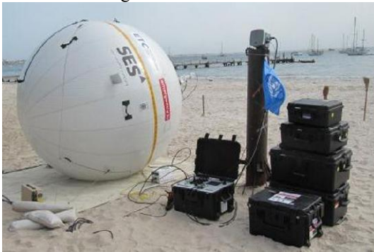
Figure 6 Emergency.lu rapid deployable kit with an inflatable satellite dish
