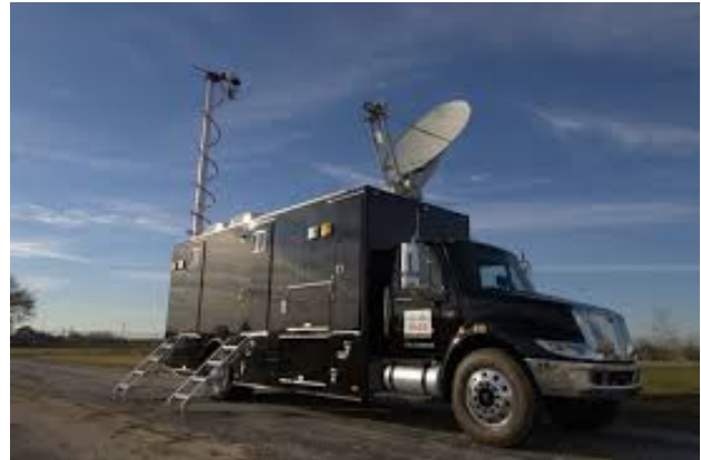
Figure 5 CISCO NERV vehicle - a complete telecommunication emergency recovery solution
