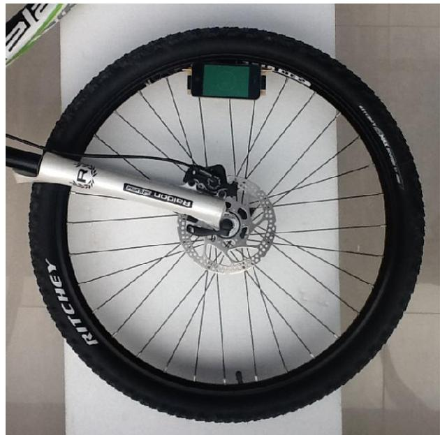
Figure 2. A horizontally balanced bicycle wheel. The smart phone is tied to the wheel. When the wheel is spun, the sensors go round the wheel's axes in a circle with the radius of  $r = 22$  cm.
