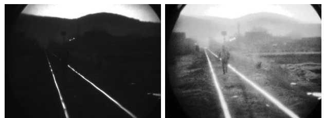
Figure 9. One of the tested scenarios with night vision system (left) [7], Image after histogram equalization (right)
