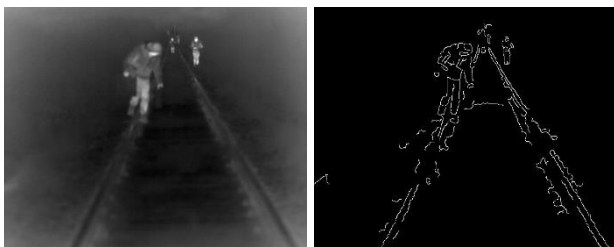
Figure 6. Tested scenario No.1 captured with IR camera at night conditions (left), Rail track detection using Canny edge detector (right) [10]
