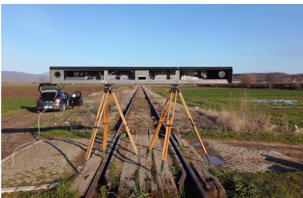
Figure 2. On-board obstacle detection system during static tests [7]
