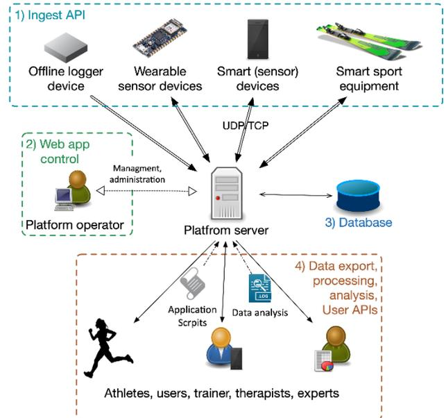
Figure 1: General architecture of the proposed platform. Most basic components can be divided into groups: 1) input devices connected to the ingest API, 2) web application for management and control, 3) relational database, and 4) post-processing and output devices.
