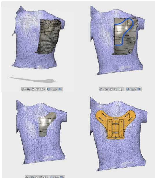
Figure 3. Modeling the "butterfly" component based on back images in Autodesk Fusion360
