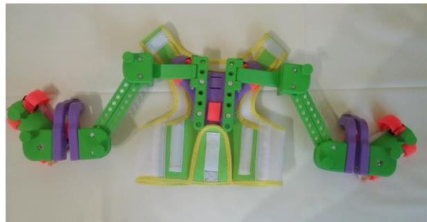
Figure 5. 3D printed customized orthosis
