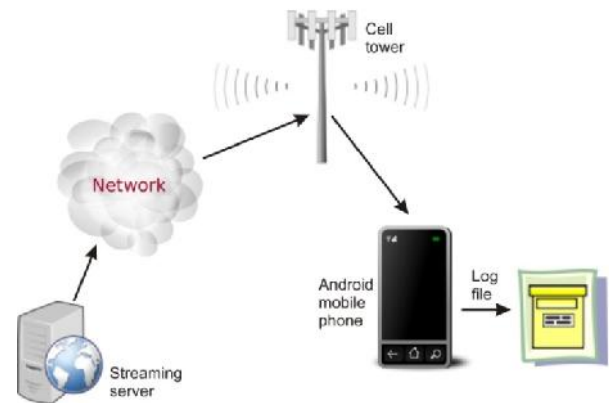
Figure 1. Architecture of the system used to record received packets
