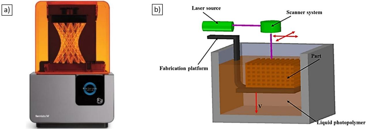
Figure 5. Showing a) by Formlabs Form 2 SLA 3D printer, b) schematic representation of a typical SLA setup [13]
