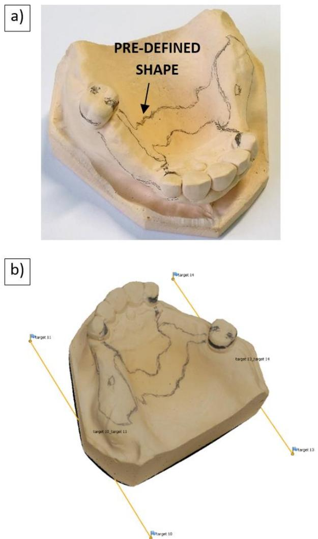
Figure 2. Showing a) dental cast with manually drawn sketches and b) 3D digitized object with applied texture in Agisoft Photoscan software
