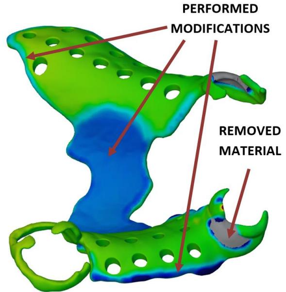
Figure 8. Color deviation showing performed modifications on the revised 3D model of RPD
