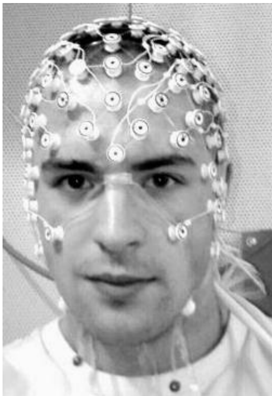
Figure 4. EEG measurement setup with electrode cap by Douglas Myers [25]
