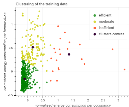
Figure 2. An illustration of three different energy efficiency clusters with their respective cluster centers (each dot represents one household's measurement obtained for a predefined time range)
