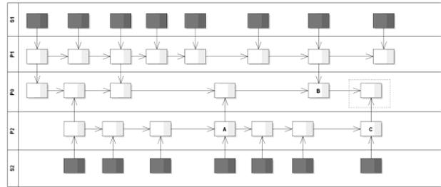
Figure 5. SysML activity diagram showing the information graph of a MSDF architecture realization for a two sensor system, with decision variables having the following values:  $V1 = 2$ ,  $V2 = \{2, 1\}$ ,  $V3 = \{CCM-H, CCM-H\}$ .
