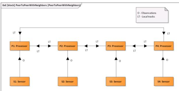
Figure 4. Example of a MSDF architecture realization for a four sensor system. Decision variables have the following values:  $V1 = 1$ ,  $V2 = \{4\}$ ,  $V3 = \{CCM-PPN\}$ .
