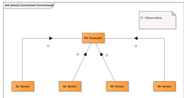
Figure 1. Example of a MSDF architecture realization for a four sensor system. Decision variables have the following values: V1 = 1, V2 = {1}, V3 = {CCM-C}.
