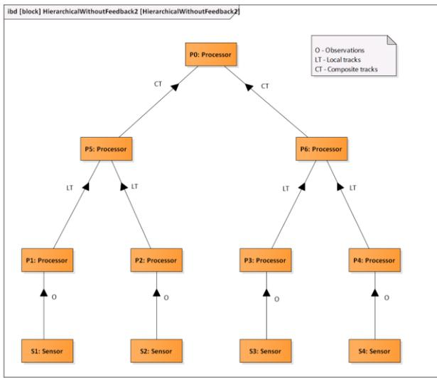
Figure 3. Example of a MSDF architecture realization for a four sensor system. Decision variables have the following values:  $V1 = 3$ ,  $V2 = \{4, 2, 1\}$ ,  $V3 = \{CCM-H, CCM-H, CCM-H\}$ .
