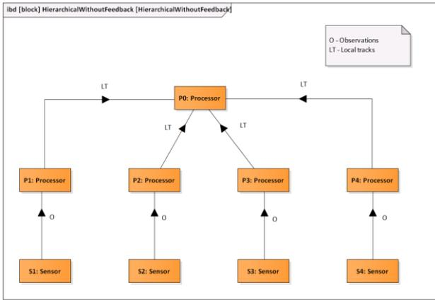
Figure 2. Example of a MSDF architecture realization for a four sensor system. Decision variables have the following values:  $V1 = 2$ ,  $V2 = \{4, 1\}$ ,  $V3 = \{CCM-H, CCM-H\}$ .
