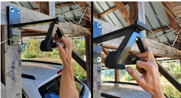
Figure 7. Conducting measurement with whole-hand open-crimp grip (left) and middle finger open-crimp grip (right).
