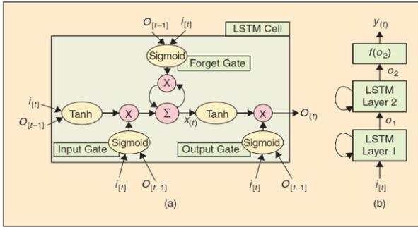
Figure 7: (a) An LSTM cell and (b) a multilayer LSTM network [15]
