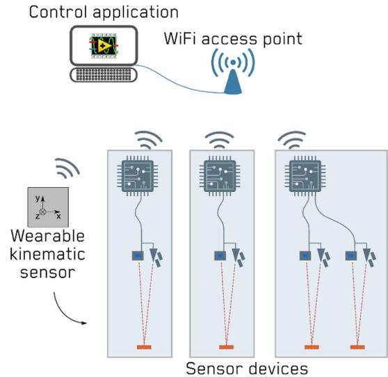
Figure 2 Architecture of the system. Devices and sensors are connected to the LabVIEW control application via Wireless access point. Wearable kinematic sensor is mounted on the athlete. Optical gates are located at specific positions as required by the test. Each sensor device can support one or multiple optical gates.
