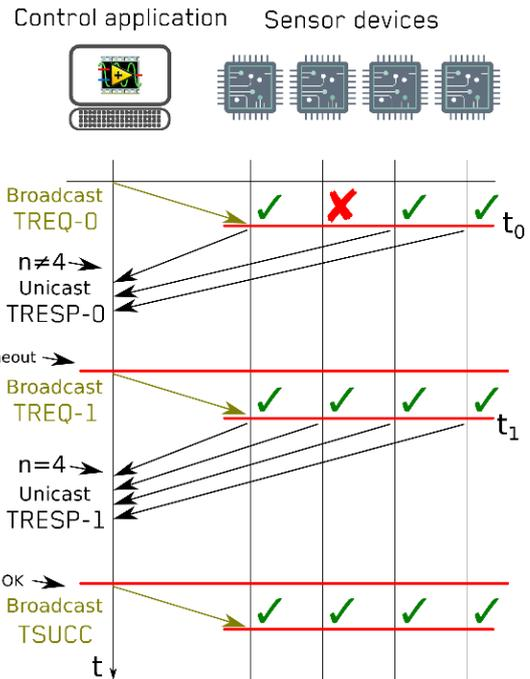
Figure 3 Synchronization protocol diagram. Server sends request (TREQ- $m$ ) to all the devices on the same network using a broadcast address. Devices respond with TRESP- $m$  message. If server does not receive the response from all the devices, it starts the synchronization cycle  $m+1$ . When all devices successfully confirm the synchronization, the server broadcast a successful sync message (TSUCC) indicating to the devices, they can start streaming data.
