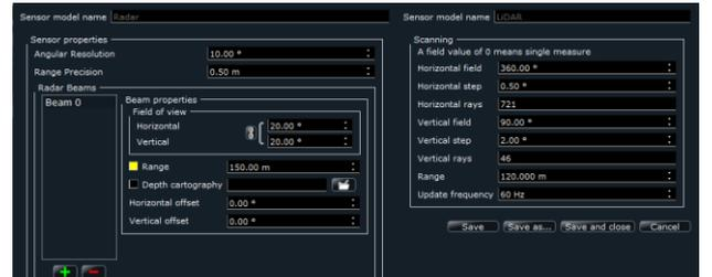
Figure 3: Configuration parameters for radar meter and LIDAR.
