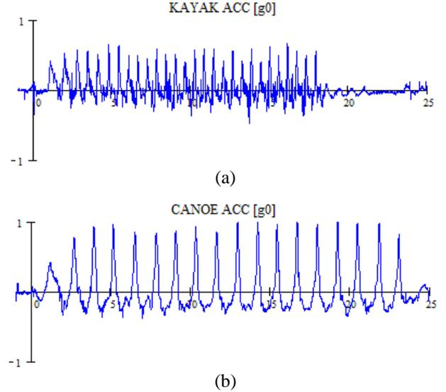
Figure 6. Boat acceleration signal in kayaking (a) and canoeing (b).
