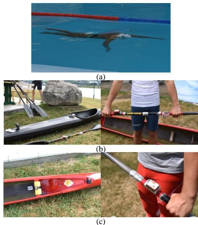
Figure 1. Placement of sensor for different water sports. (a) Swimming: the movement of the body is detected by a sensor in the belt strapped to the lower back (b). Kayaking: sensors are attached to the top of the kayak and to the paddle. (c) Canoeing: sensors are attached to the bottom of the canoe and to the paddle.
