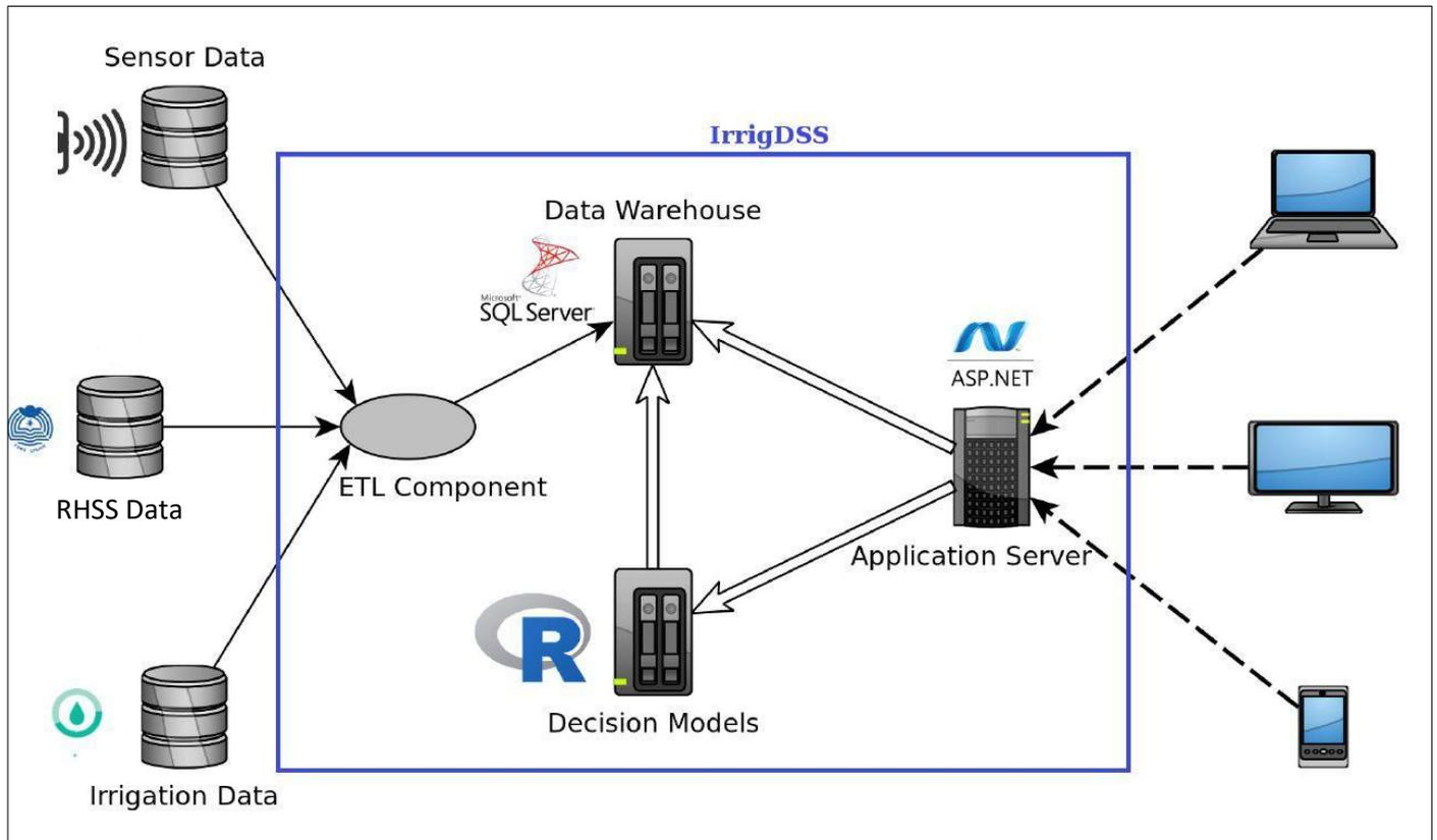
Figure 1 – Overview of the IrrigDSS architecture
