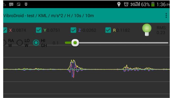
Figure 2. Measuring vibrations using the VibroDroid application
