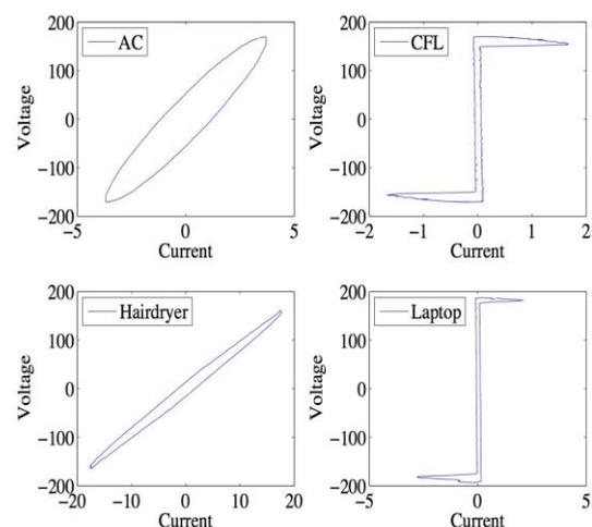
Figure 1. Examples of V-I trajectories
