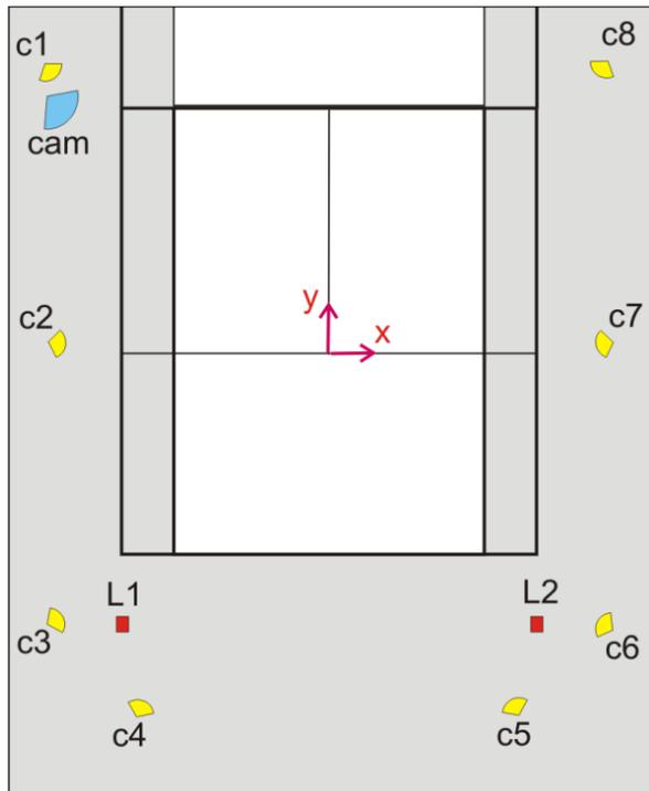
Figure 2. Localization systems field setup: (a) Eight Qualisys cameras (c1-c8) are covering half of tennis court, two UWB anchors are located behind the court (L1, L2), and a wide angle video camera (cam) is positioned near c1.
