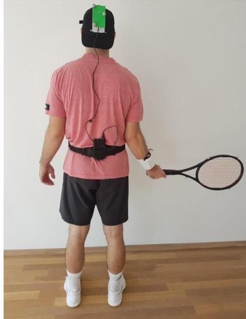
Figure 1. Attachment of wearable sensors and reflective markers. UWB tag is attached to the cap, ball impacts are detected by a sensor attached to the wristband, battery is attached to the belt. For the optical tracking system, the UWB device position object is defined by three reflective markers and the tennis racket is defined as a solid object with four reflective markers with the origin in the racket head center.
