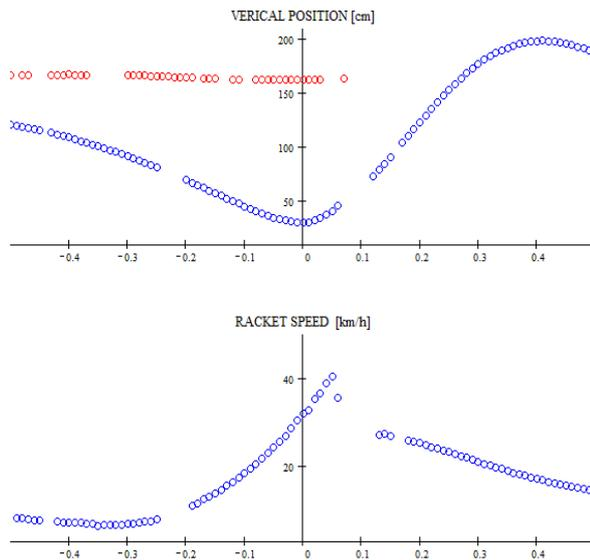
Figure 3. Some additional parameters can be precisely acquired by the optical tracking system. (top) Tennis racket center (blue) and players head (red) distance to ground [cm]. (bottom) Tennis racket center velocity vector magnitude around the impact [km/h].
