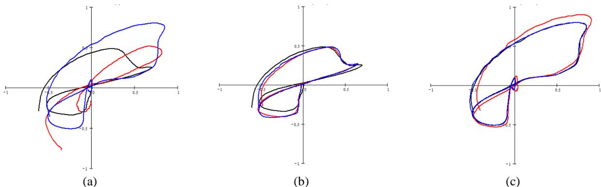
Figure 3. Smart golf club prototype includes a 2D bending sensor; its trajectories confirm high consistency of players swings. Average trajectories (N=10) show (a) large differences between three different players' signatures, and much smaller differences between the perfect swing and faulty swings of the same player (b) and (c).
