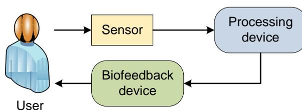
Figure 1. General architecture of a biofeedback system.
