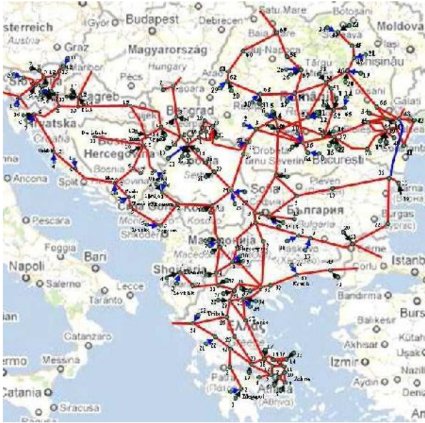
Figure 1. Electric power grid of Southeast Europe
