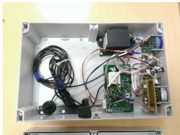
Figure 3. ekoNET device with low-cost electrochemical gas sensors
