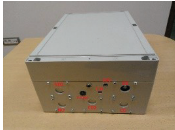
Figure 2. ekoNET device with low-cost electrochemical gas sensors mounted in the box
