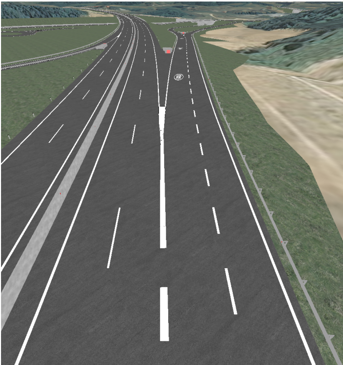
Fig. 6. Optimized model in Blender: decimated terrain surface, added road markings, guardrails with reflectors and supporters, deer fences, and crumple zones.
