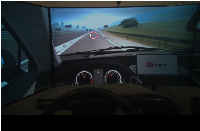
Fig. 7. Driver's gaze during the evaluation of a road segment.
