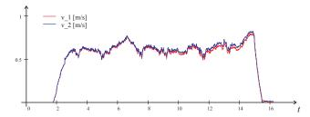
Figure 5. Smart phone velocity  $v_y$  in the direction of Y axis. The velocity  $v_y$  is calculated by: (a) algorithm 1  $(v_1)$ , which uses accY data that gives us the acceleration in the direction of movement and gyroZ data that gives us the information about smart phone orientation in the (x,y) plane, (b) algorithm 2  $(v_2)$  uses the accX and accY data to directly calculate the velocity  $v_y$ .
