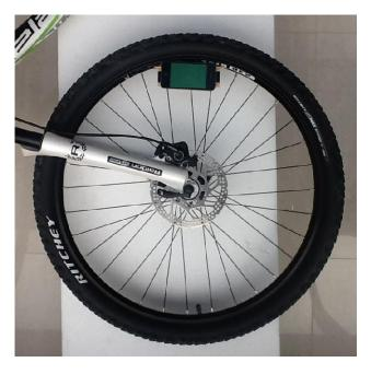
Figure 2. A horizontally balanced bicycle wheel. The smart phone is tied to the wheel. When the wheel is spinned, the sensors go round the wheel's axes in a circle with the radius of r=22 cm.
