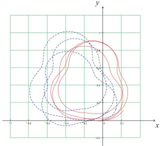
Figure 8. Calculated trajectory of the smart phone movement on the inner track from Figure 1. The solid curve shows the trajectory calculated by the algorithm 1 and the dashed curve shows he trajectory calculated by the algorithm 2. We notice that the results obtained by fusing the accelerometer and gyroscope data (algorithm 1) give much more faithful trajectory.
