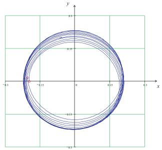
Figure 9. Calculated trajectory of the smart phone movement on the bicycle wheel 2. The trajectory is calculated by algorithm 1. We see that the iPhone makes circles with the radius of about r=22 cm, what faithfully represents the conditions of the test.
