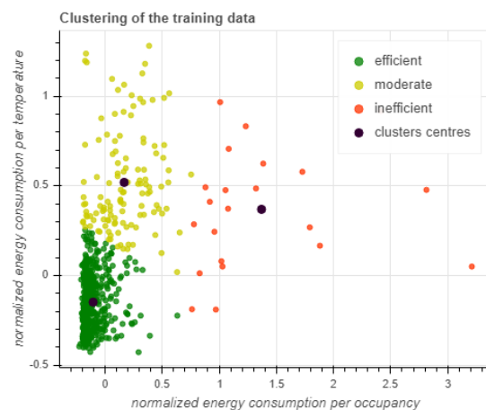
Figure 2. An illustration of three different energy efficiency clusters with their respective cluster centers (each dot represents one household's measurement obtained for a predefined time range)
